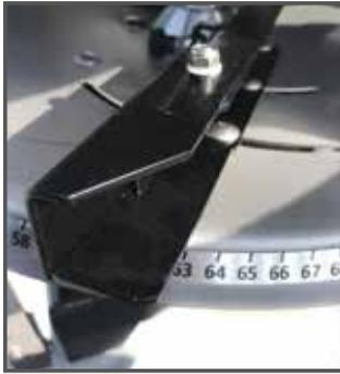
MT-vanes can be accurately adjusted in length and orientation from 18 to 36 metres according to the type of fertiliser, seeds and snail/slug pellets. The operator, thanks to the clearly visible graduations, can adjust quickly without the need for tools.
